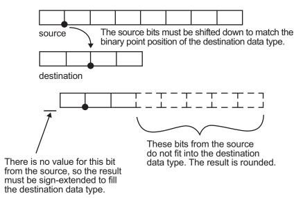
As the diagram shows, the source bits are shifted down so that the binary point matches the destination binary point position. There is no value for the highest bit from the source, so sign extension is used to fill the integer portion of the destination data type. The bottom five bits of the source do not fit into the fraction length of the destination. Therefore, precision can be lost as the result is rounded.
